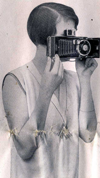
Fig. 5 How to hold the camera for a horizontal exposure when using the iconometer view finder
