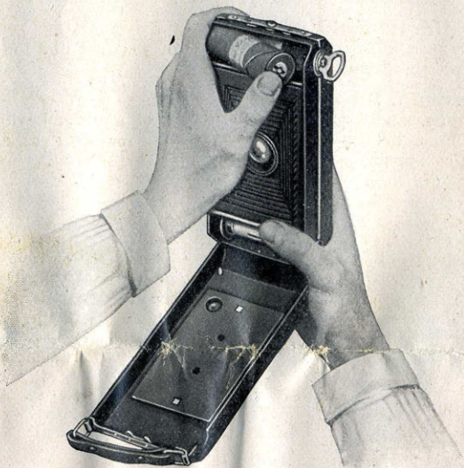
Fig. 7 Showing the method of removing the spool
